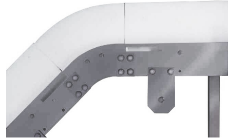
1 INCLINE TO HORIZONTAL SECTION
