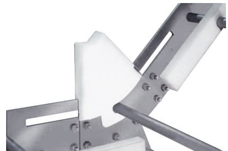
4 INCLINE BELT HOLD DOWN
