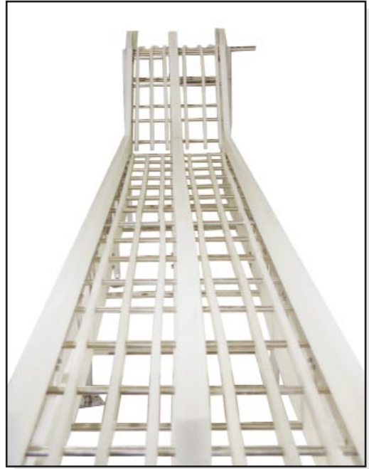
Dual lane incline conveyor with over-belt side-rails and lane dividers. Also shown are snap in place belt support rails and spanner bars.
