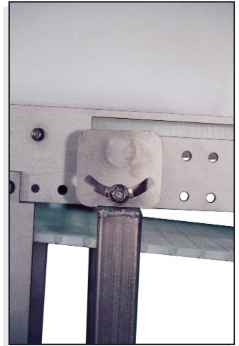
Adjustable incline leg bracket allows conveyor angle adjustment up to 45 degrees.
