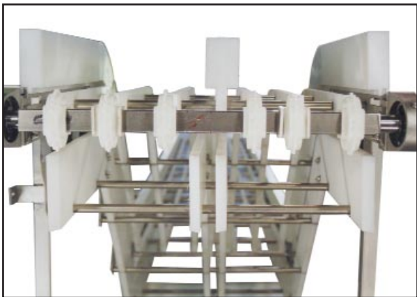
End view of conveyor frame, over-belt side-rails and lane divider.
